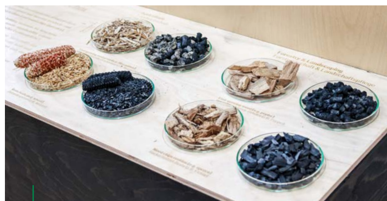
Four different types of plant-based charcoal on display, each made from distinct raw materials: straw and grass, fast-growing wood, corn and wheat husks, and wood chips (from left to right, top to bottom)
